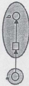
Figure 17: The trap \{a, b\} is not strongly connected; its image is not a trap of the target net
