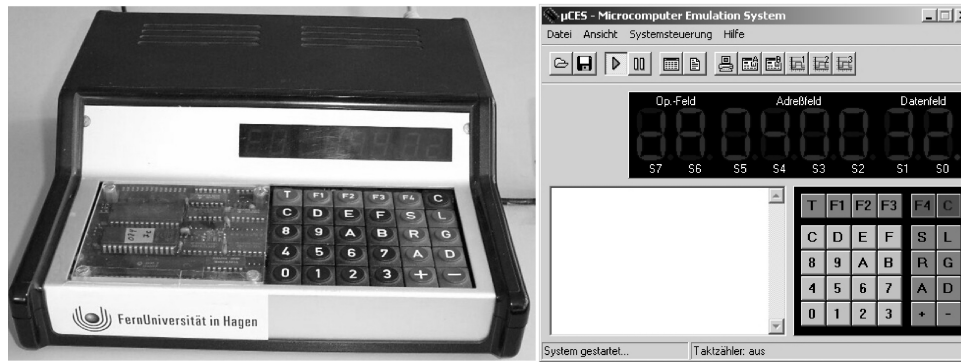
Figure 9. The real microcomputer (left) and the graphical interface of its simulator/remote control (right).
