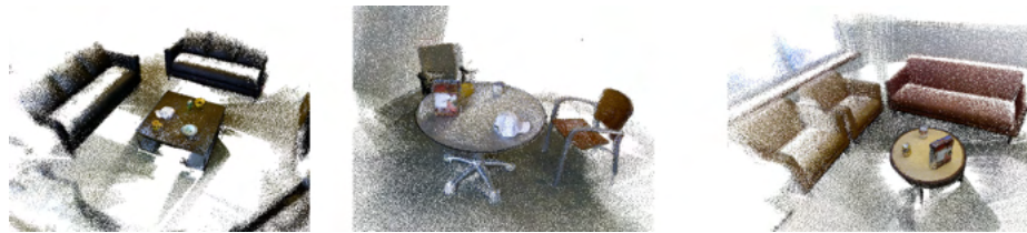
Figure 7.7: Point clouds of Trimble 3D Warehouse [44] objects as part of the RGB-D Scenes Dataset v.2. The dataset contains segmented objects in 9 categories placed in different scenes to evaluate object recognition systems.
