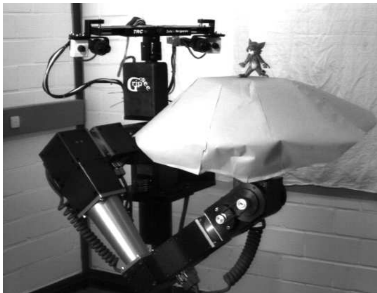
Figure 2.1: Robot Scene. The robot arm has object “Tom” fixed in its gripper. The gripper itself is covered by a gray background.
