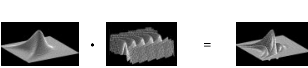
Figure 5: The real part of a banana wavelet is the product of a curved Gaussian G^{\vec{b}}(x, y) and a curved wave function F^{\vec{b}}(x, y) .
