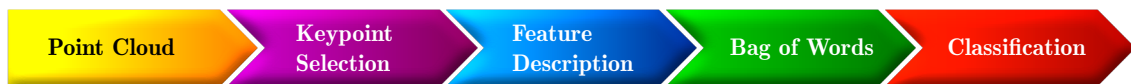
Figure 2: The classification pipeline used for the evaluation of local 3-D feature descriptors. It consists of four main steps: keypoint selection, feature descriptions, a bag-of-words model, and the classification.
