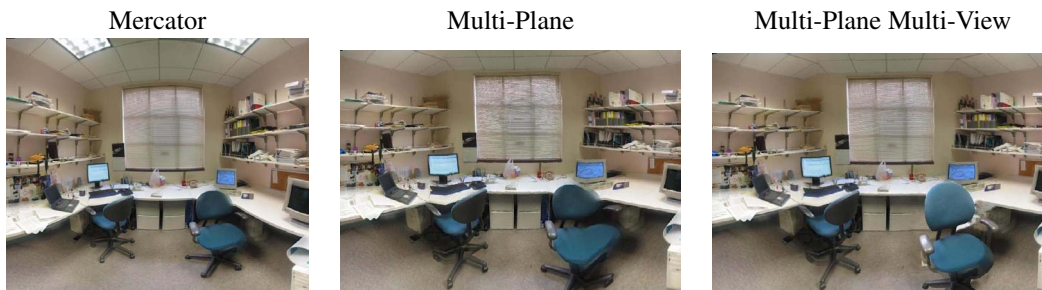
Figure 9. Multi-Plane Multi-View. The multi-plane projection rectified the background but the chair on the right got distorted. Using the Multi-View approach the chair is undistorted.
